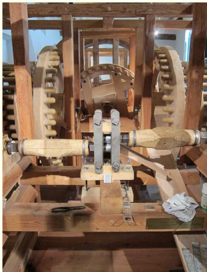
Fig. 3: Roller press minting was invented in Zurich and perfected in Hall. The roller press depicted here is a reconstruction that can be admired in Hall. Photo: KW.
