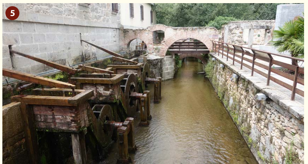
The water turns the mill wheel, which in turn sets the roller presses in motion. Photo: UK.
